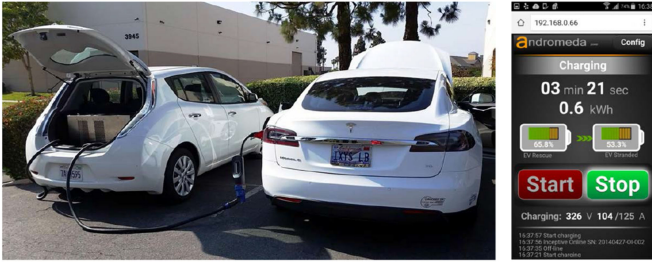
Fig. 1. A Nissan Leaf is transferring energy to a Tesla Model S through a conductive charging cable. A mobile app communicating with both vehicles lets the drivers control the charging process [6], [18].
