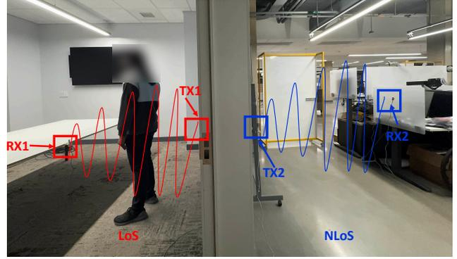
Fig. 2: Experimental setup for LoS and NLoS scenarios
