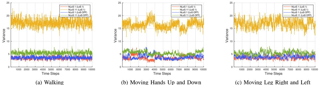
Fig. 4: Variance of amplitude across subcarriers during all repetitions of each activity for NLoS pairs of Experiment 1.
