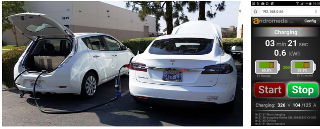
Fig. 1. A Nissan Leaf is transferring energy to a Tesla Model S through a conductive charging cable. A mobile app communicating with both vehicles lets the drivers control the charging process [24], [26]
